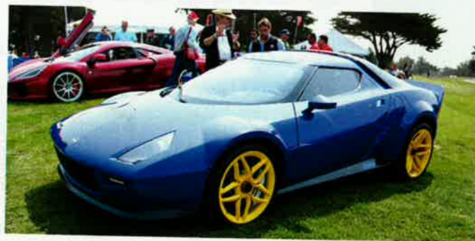
Making the show rounds worldwide over the past couple of years, this carbon-fiber-bodied neo Stratos, inspired by the original Lancia rally-dominating machine from the 1970s, is built on a highly modified Ferrari 430. The donor car lost several inches of wheelbase during the conversion process carried out by Manifattura Automobili Torino.
